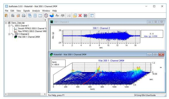
Figure 3: Signal list window with two signals and computed results (left) and plot window with time history and Waterfall plots (right)
