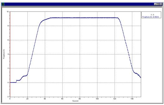
This plot is the raw DC tachometer signal.
