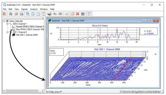
Figure 20: Slide the "Smooth RPM" from signal list to Waterfall to add Speed data to the Waterfall
