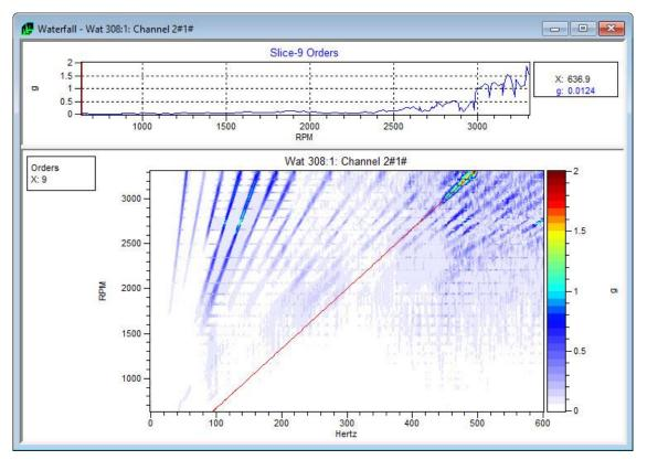
Figure 51: Contour Plot as function of RPM with "order cursor" at order 9
