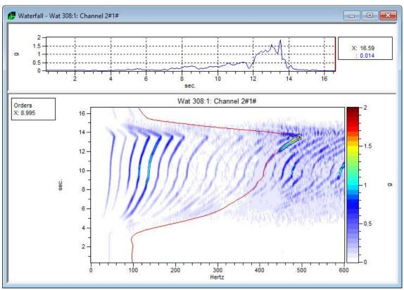
Figure 50: Contour Plot as function of time with "order cursor" at order = 8.995
