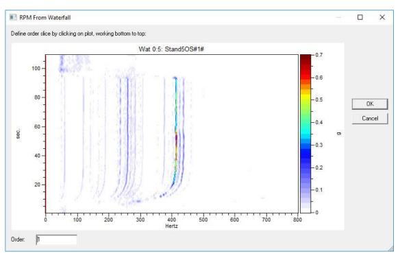
Figure 30: RPM from Waterfall dialog window
