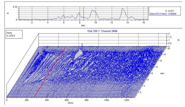
**4.** ibaRotate displays the acceleration waterfall, and the slice at the cursor:
