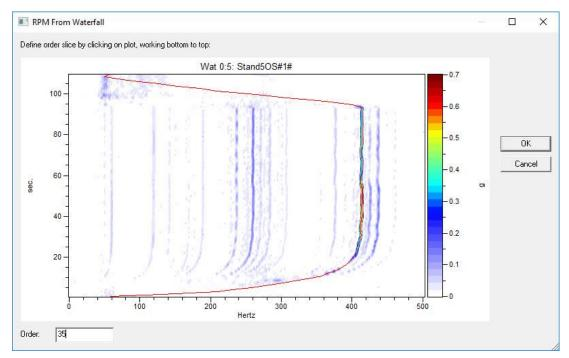
Figure 32: Order selection line on contour plot in the RPM from waterfall dialog window
