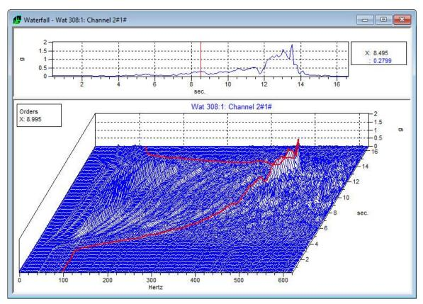
Figure 49: Waterfall with "Order cursor" positioned on the response ridge at order = 8.955
