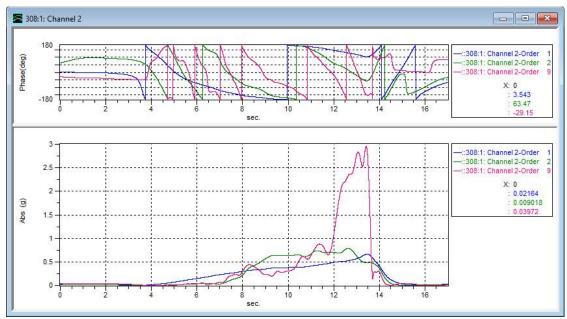
Figure 37: Complex envelopes by Vold-Kalman filter
