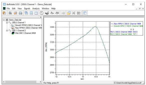
Figure 19: Signal list window contains data from tachometer processing
