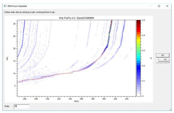
Figure 31: Zoom of contour on RPM from waterfall dialog window
